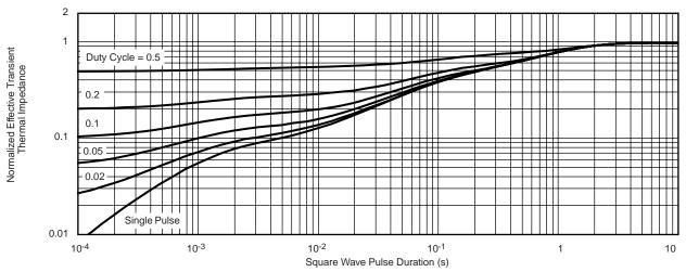
Normalized Thermal Transient Impedance, Junction-to-Foot
