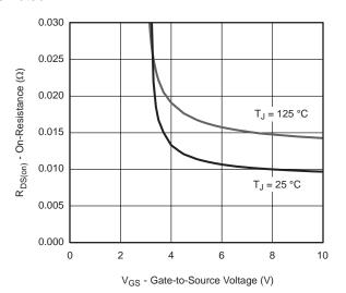
On-Resistance vs. Gate-to-Source Voltage
