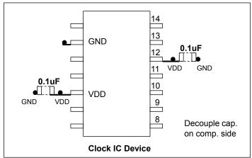
Placement of Decoupling Capacitors
