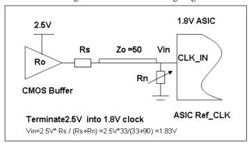
Rs =  $33\Omega$  with Rn =  $100\Omega$ , to transition 3.3V CMOS to 2.5V
