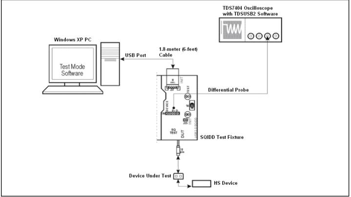
Figure 1: HS Eye Test Setup
