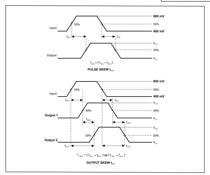
Figure 7. Skew Test
