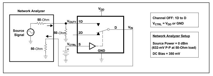
Figure 3. OFF Isolation (O<sub>ISO</sub>)
