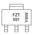
FZT 591 = Product Type Marking Code YWW = Date Code Marking Y or  $\overline{Y}$  = Last Digit of Year (ex: 2 = 2022) WW or  $\overline{W}W$  = Week Code (01 to 53)
