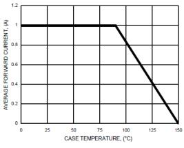
FIG.1- FORWARD CURRENT DERATING CURVE
