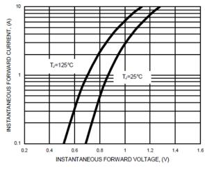
FIG.3- TYPICAL FORWARD CHARACTERISTICS
