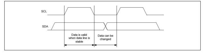
\*Note with caution that if the SDA data is changed while the SCL line is at high level, it will be treated as a START, RESTART, or STOP condition.
