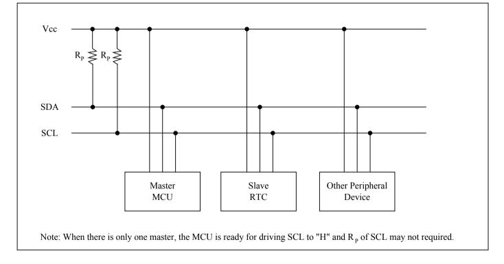
Fig 1. System configuration
