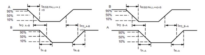
Figure 4. Definition of Timing Specification Parameters
