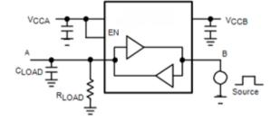
Figure 2. Driving A Test Circuit
