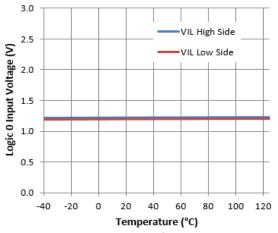
Figure 24. Logic 0 Input Voltage vs. Temperature
