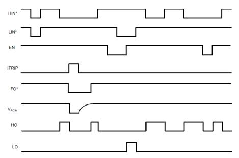
Figure 2. Input/Output Timing Diagram
