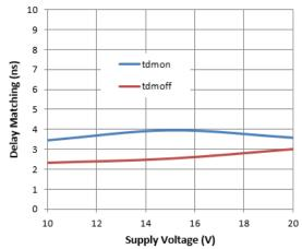
Figure 15. Delay Matching vs. Supply Voltage
