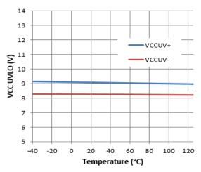
Figure 25. VCC UVLO vs. Temperature
