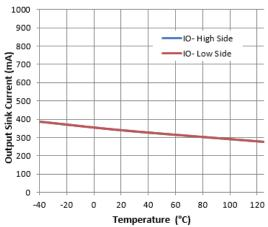
Figure 20. Output Sink Current vs. Temperature
