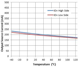
Figure 18. Output Source Current vs. Temperature
