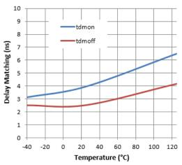
Figure 16. Delay Matching vs. Temperature
