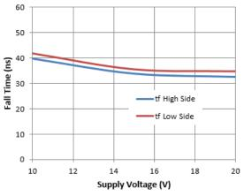
Figure 11. Fall Time vs. Supply Voltage
