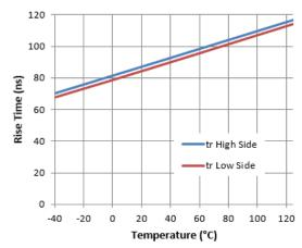
Figure 10. Rise Time vs. Temperature
