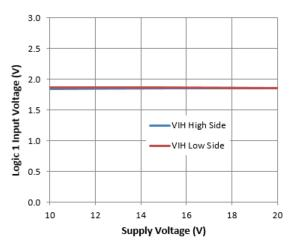
Figure 21. Logic 1 Input Voltage vs. Supply Voltage
