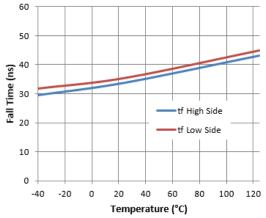
Figure 12. Fall Time vs. Temperature
