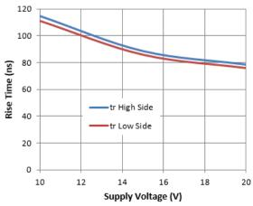
Figure 9. Rise Time vs. Supply Voltage
