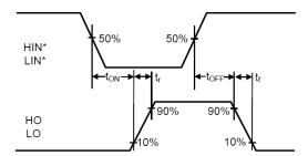
Figure 1. Switching Time Waveform Definitions
