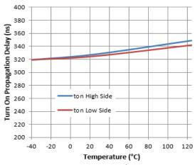
Figure 6. Turn-on Propagation Delay vs. Temperature
