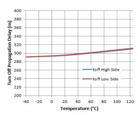
Figure 8. Turn-off Propagation Delay vs. Temperature
