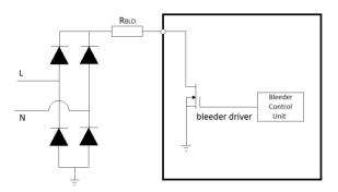
Figure 3. Internal Bleeder Circuitry
