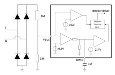
Figure 4. Phase angle and dimmer Detection
