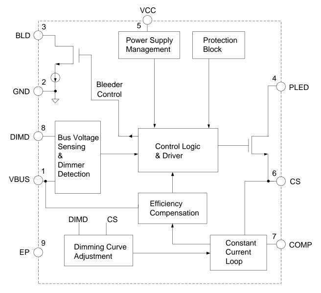
Figure 2. AL5892 Functional Block Diagram
