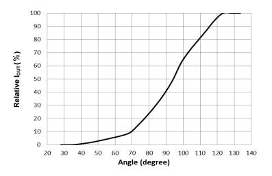
Figure 7. Relative LED Current vs. TRIAC Phase Angle
