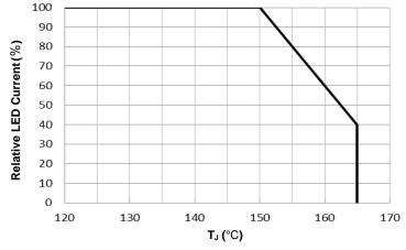
Figure 6. Thermal Fold Back
