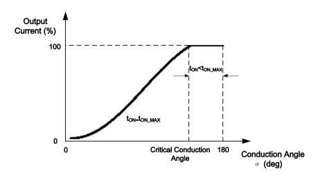
Figure 2. Dimming Curve
