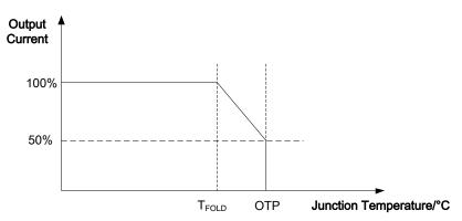
Figure 1. Thermal Foldback Waveform
