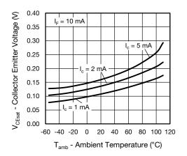
Fig. 11 - Collector Emitter Voltage vs. Ambient Temperature
