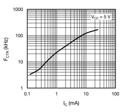
Fig. 15 - F<sub>CTR</sub> vs. Collector Current
