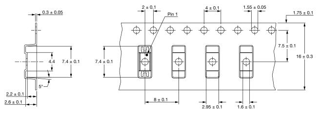
Fig. 18 - Tape and Reel Packing (3000 parts per reel)
