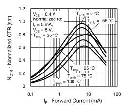
Fig. 13 - Normalized CTR (saturated) vs. Forward Current
