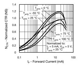
Fig. 12 - Normalized CTR (non-saturated) vs. Forward Current
