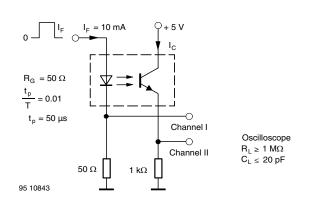
Fig. 2 - Test Circuit, Saturated Operation
