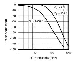
Fig. 14 - F<sub>CTR</sub> vs. Phase Angle
