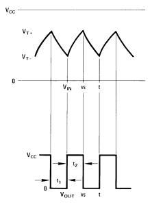
$$f \approx \frac{1}{\text{RC In} \frac{V_T + (V_{CC} - V_{T-})}{V_T - (V_{CC} - V_{T+})}}$$
