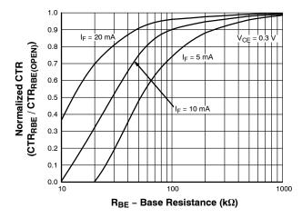
Figure 5. CTR vs. RBE (Saturated)
