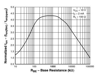
Figure 8. Normalized ton vs. RBE
