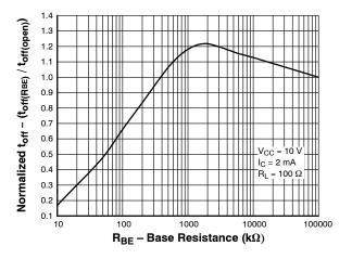
Figure 9. Normalized  $t_{\text{off}}$  vs.  $R_{\text{BE}}$
