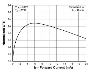
Figure 2. Normalized CTR vs. Forward Current
