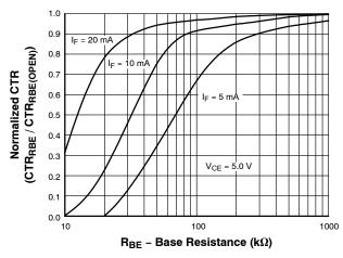
Figure 4. CTR vs. RBE (Unsaturated)
