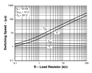
Figure 7. Switching Speed vs. Load Resistor
