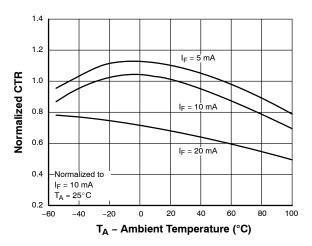
Figure 3. Normalized CTR vs. Ambient Temperature
