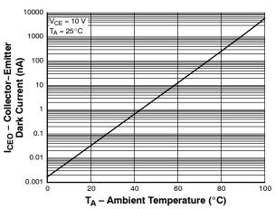
Figure 10. Dark Current vs. Ambient Temperature
