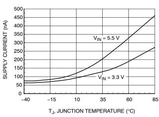
Figure 6. I<sub>SHUTDOWN</sub> Current vs. Temperature
