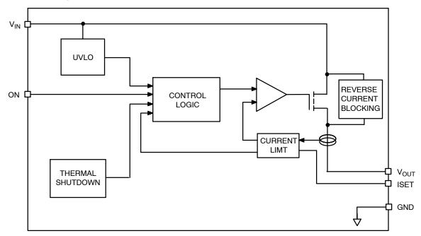
Figure 2. Block Diagram
