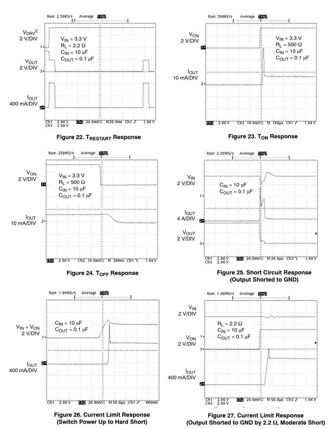
NOTE:  $V_{DRV}$  signal forces the device to go into overcurrent condition by loading a 2.2  $\Omega$  resistor.
