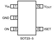
Figure 3. Pin Assignment
