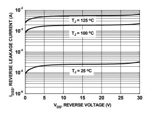
Figure 15. SyncFET<sup>TM</sup> Body Diode Reverses Leakage vs. Drain-Source Voltage
