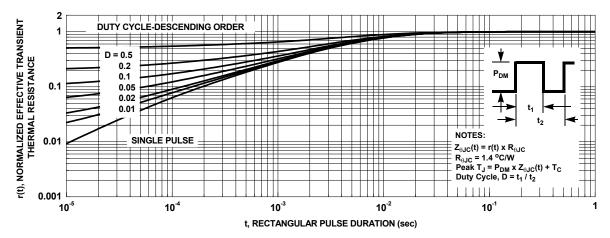
Figure 13. Junction-to-Case Transient Thermal Response Curve
