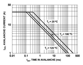
Figure 9. Unclamped Inductive Switching Capability
