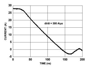
Figure 14. FDMS7658AS SyncFET<sup>TM</sup> Body Diode Reverse Recovery Characteristic
