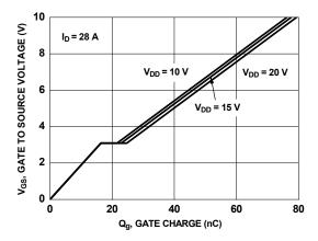
Figure 7. Gate Charge Characteristics
