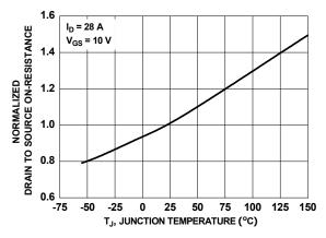
Figure 3. Normalized On-Resistance vs. Junction Temperature
