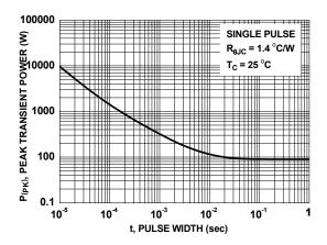
Figure 12. Single Pulse Maximum Power Dissipation
