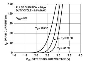
Figure 5. Transfer Characteristics
