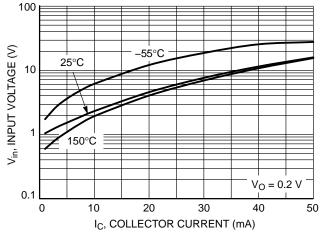
Figure 6. Input Voltage vs. Output Current
