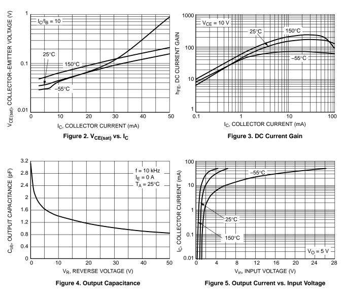
TYPICAL CHARACTERISTICS MUN2234, MMUN2234L, MUN5234, DTC124XE, DTC124XM3
