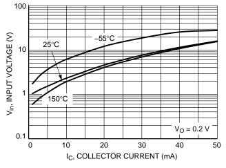
Figure 6. Input Voltage vs. Output Current
