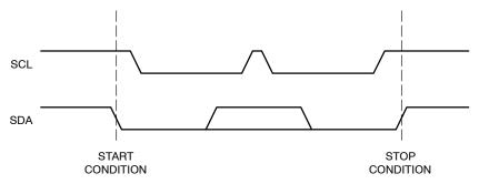
Figure 2. Start/Stop Timing
