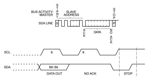
Figure 10. Immediate Address Read Timing
