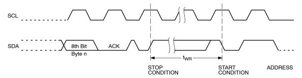
Figure 7. Write Cycle Timing
