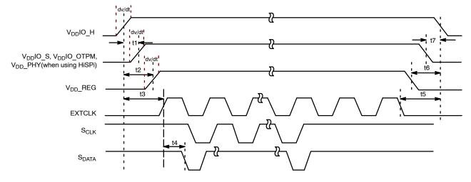
Figure 5. Power–Up and Power–Down Sequence
