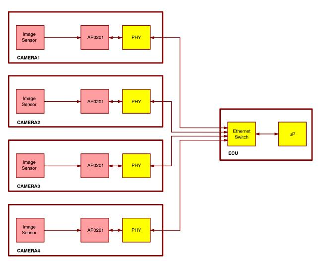
NOTE: The AP0201AT example above shows the PHY which is used between the Ethernet switch and the AP0201AT.
