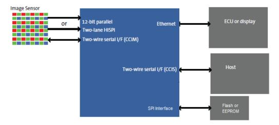
NOTE: The Hybrid mode supports configuring the AP0201AT through the serial interface and streaming video over Ethernet. Hybrid Mode can be enabled by loading an available patch. Please contact ON Semiconductor support.
