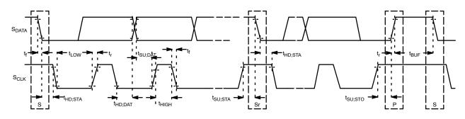
Figure 17. Master Two Wire Serial Bus Timing Parameters (CCIM)
