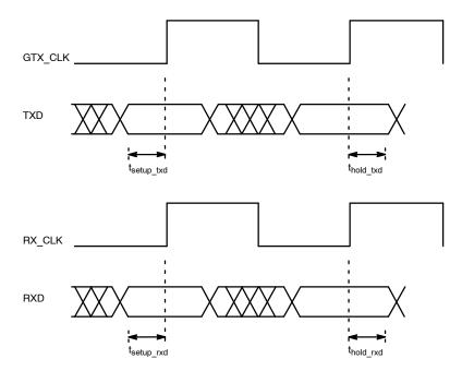
Figure 15. GMII I/O Timing Diagram
