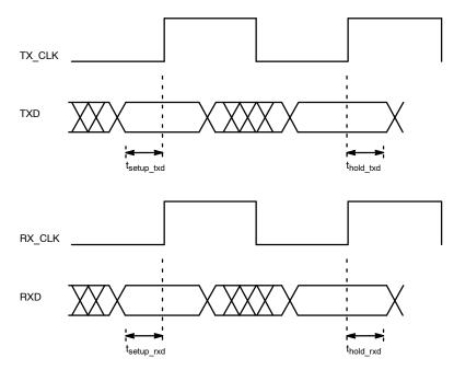
Figure 13. MII I/O Timing Diagram
