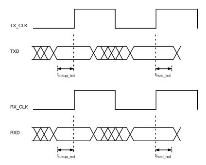
Figure 14. RMII I/O Timing Diagram
