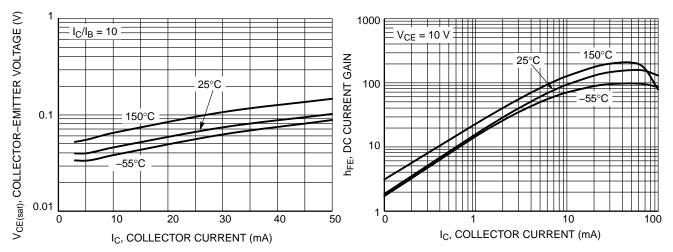
Figure 2. V<sub>CE(sat)</sub> vs. I<sub>C</sub>
