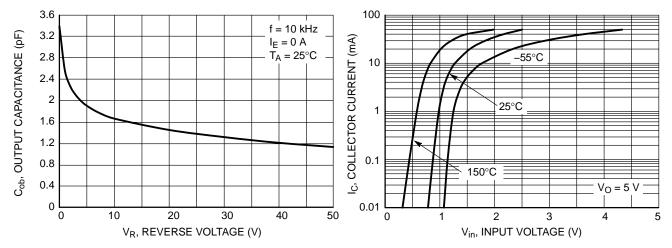
Figure 4. Output Capacitance
