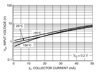
Figure 6. Input Voltage vs. Output Current
