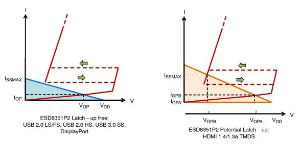
Figure 7. Example Load Lines for Latch-up Free Applications and Applications with the Potential for Latch-up
