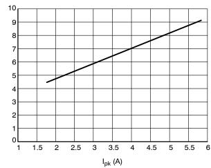
Figure 2. Clamping Voltage vs Peak Pulse Current (  $t_p$  = 8/20  $\mu$ s)
