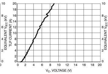
Figure 6. Negative TLP I-V Curve
