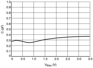
Figure 1. CV Characteristics
