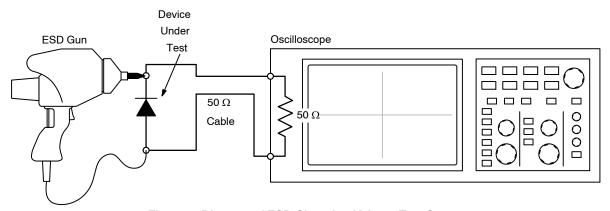
Figure 9. Diagram of ESD Clamping Voltage Test Setup
