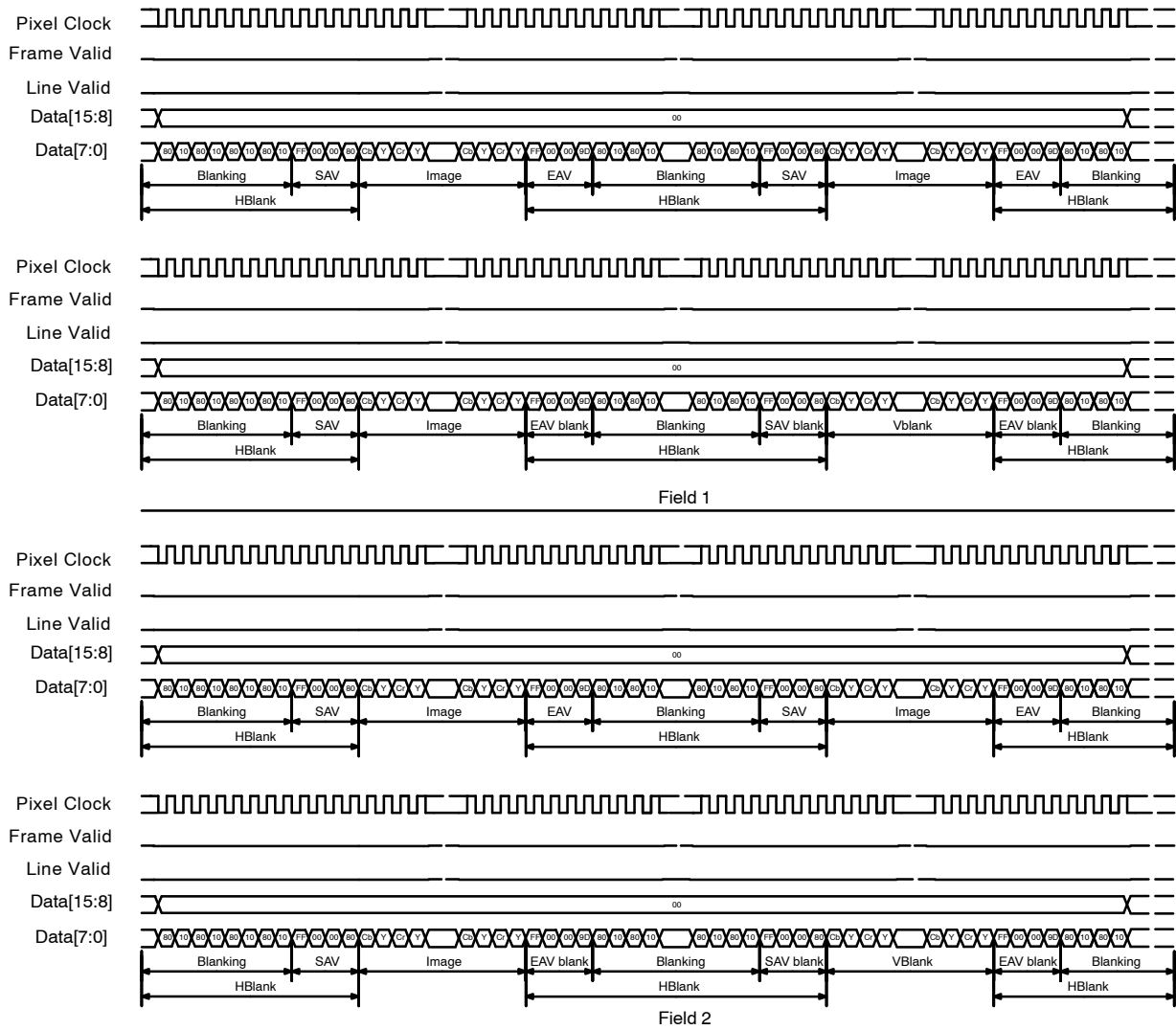
Figure 18. Typical CCIR656 Output
