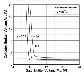
**Figure 2. Typical Output Characteristics**
