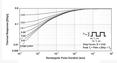
Figure 22. Transient Thermal Impedance of Diode
