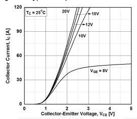
Figure 3. Typical Saturation Voltage Characteristics
