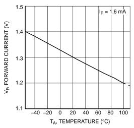
Figure 6. LED Forward Current vs. Temperature
