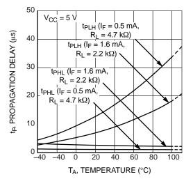
Figure 13. Propagation Delay vs. Temperature (6N138M / 6N139M Only)
