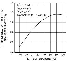
Figure 8. Normalized Current Transfer Ratio vs. Ambient Temperature (6N138M / 6N139M Only)
