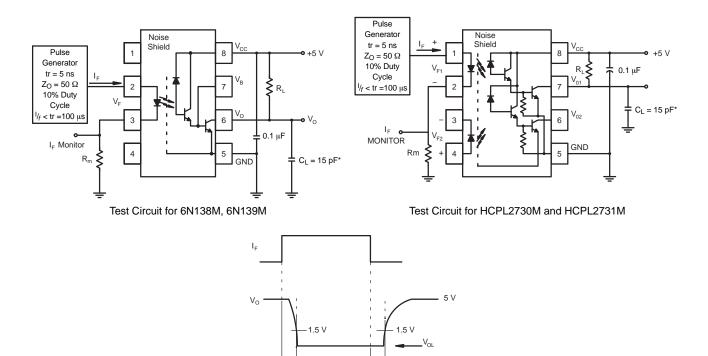
Figure 14. Switching Time Test Circuit
