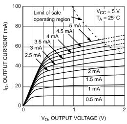
Figure 11. Output Current vs Output Voltage (6N138M / 6N139M Only)
