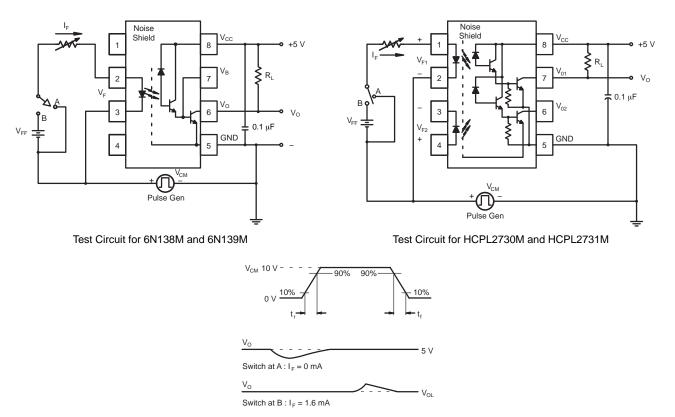
Figure 15. Common Mode Immunity Test Circuit
