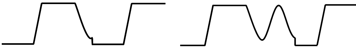
Figure 63. Full-load Operation – Quasi-resonant Mode in low line (left), turn on at valley 2 when in high line (right)
