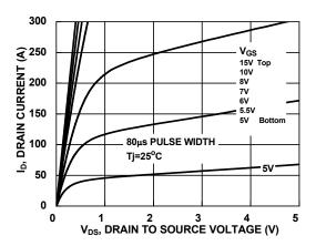
Figure 9. Saturation Characteristics
