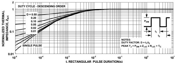
Figure 3. Normalized Maximum Transient Thermal Impedance
