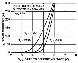
Figure 7. Transfer Characteristics
