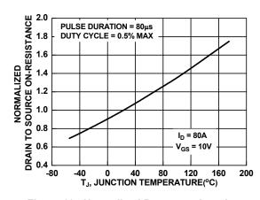
Figure 12. Normalized R<sub>DSON</sub> vs. Junction Temperature
