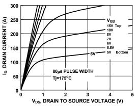
Figure 10. Saturation Characteristics
