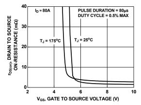
Figure 11. R<sub>DSON</sub> vs. Gate Voltage
