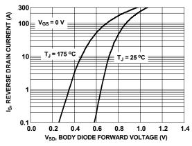
Figure 8. Forward Diode Characteristics
