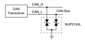
Figure 15. CAN ESD Circuit
