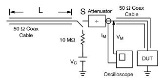
Figure 13. Simplified Schematic of a Typical TLP System
