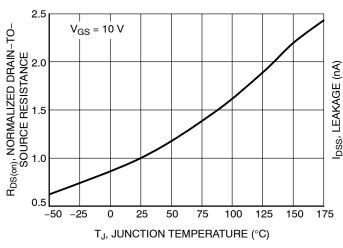
Figure 5. On–Resistance Variation with Temperature
