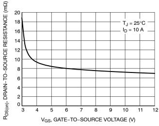
Figure 3. On-Resistance vs. Gate-to-Source Voltage
