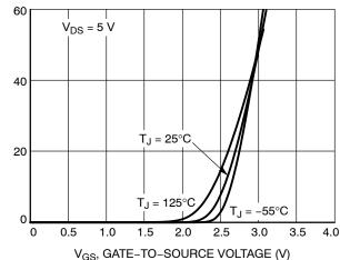
Figure 2. Transfer Characteristics
