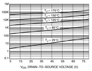
Figure 6. Drain-to-Source Leakage Current vs. Voltage
