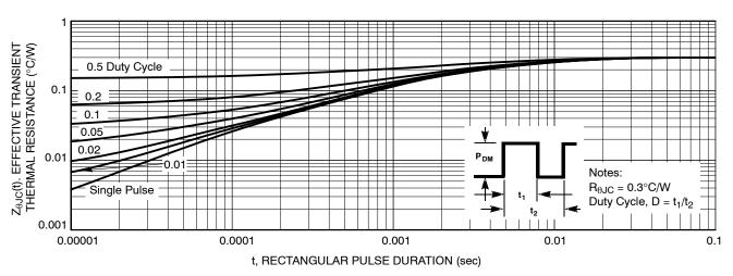
Figure 13. Junction-to-Case Thermal Response
