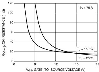
Figure 4. On-Resistance vs. Gate-to-Source Voltage
