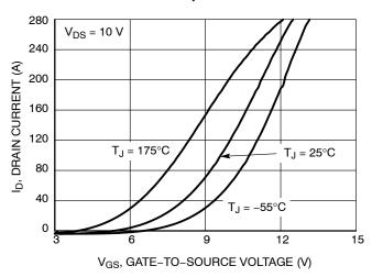
Figure 5. Transfer Characteristics
