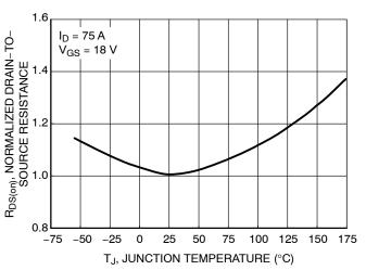
Figure 3. On–Resistance Variation with Temperature
