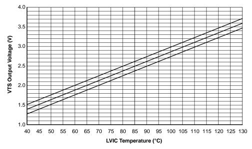
Figure 4. Temperature of LVIC versus VTS Characteristics
