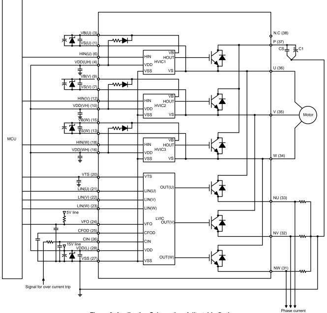
Figure 2. Application Schematic – Adjustable Option
