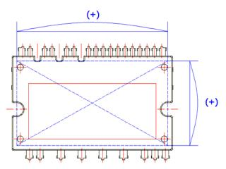
Figure 7. Flatness Measurement Position
