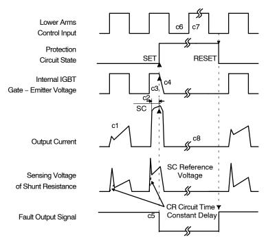
(with the external sense resistance and RC filter connection)
