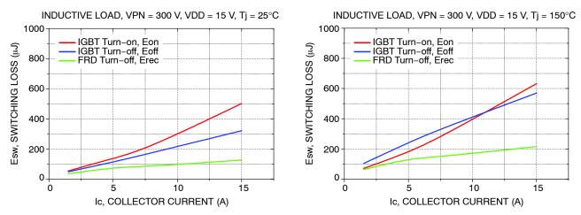
Figure 4. Switching Loss Characteristics (Typical)
