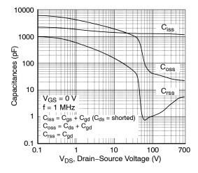
Figure 5. Capacitance Characteristics
