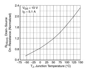
Figure 8. On-Resistance Variation vs. Temperature
