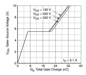
Figure 6. Gate Charge Characteristics
