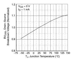
Figure 7. Breakdown Voltage Variation vs. Temperature
