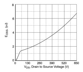
Figure 11.  $E_{\text{OSS}}$  vs. Drain to Source Voltage
