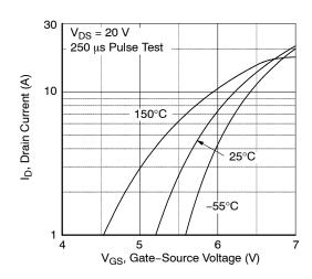
Figure 2. Transfer Characteristics
