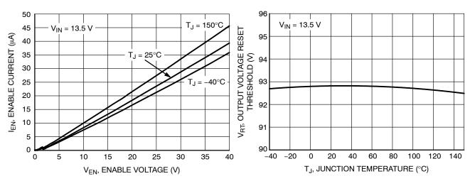
Figure 28. Enable Current vs. Enable Voltage
