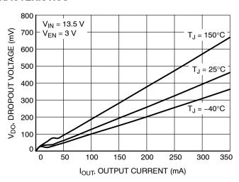
Figure 11. Dropout vs. Output Current (5 V Option)
