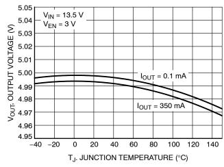
Figure 7. Output Voltage vs. Temperature (5 V Option)
