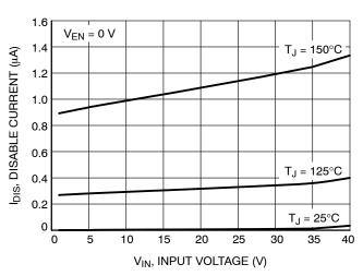
Figure 27. Disable Current vs. Input Voltage
