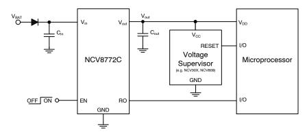
Figure 34. Application Diagram
