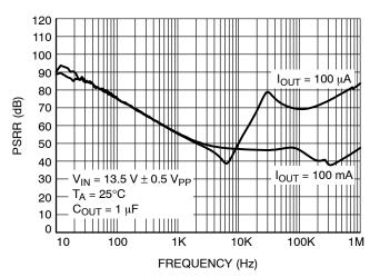
Figure 23. PSRR vs. Frequency (3.3 V Option)
