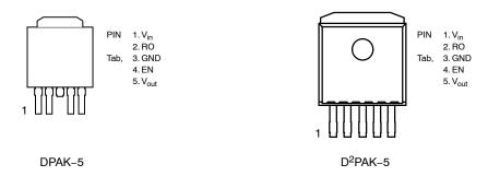
Figure 3. Pin Connections
