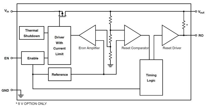
Figure 2. Simplified Block Diagram
