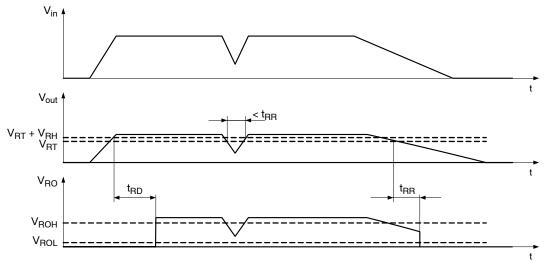
Figure 31. Reset Function and Timing Diagram
