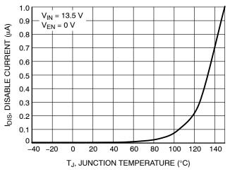
Figure 26. Disable Current vs. Temperature
