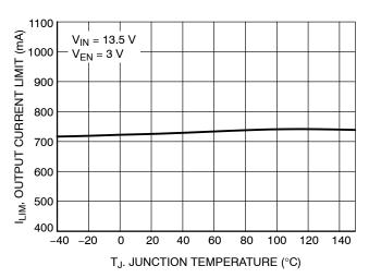
Figure 15. Output Current Limit vs. Temperature
