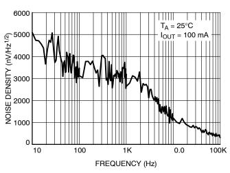
Figure 24. Noise vs. Frequency
