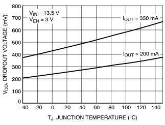
Figure 12. Dropout vs. Temperature (5 V Option)
