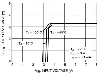
Figure 10. Output Voltage vs. Input Voltage (3.3 V Option)
