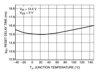
Figure 30. Reset Delay Time vs. Temperature
