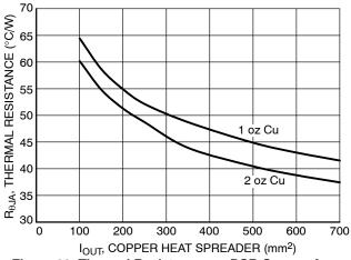
Figure 32. Thermal Resistance vs. PCB Copper Area (D2PAK-5)
