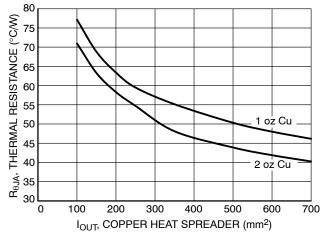
Figure 33. Thermal Resistance vs. PCB Copper Area (DPAK-5)
