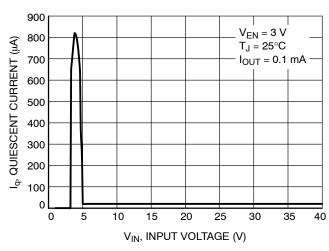
Figure 5. Quiescent Current vs. Input Voltage
