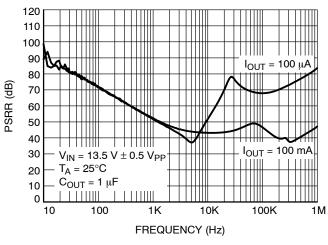
Figure 22. PSRR vs. Frequency (5 V Option)
