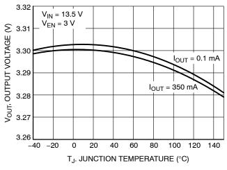
Figure 8. Output Voltage vs. Temperature (3.3 V Option)
