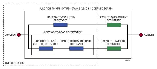
Figure 3. Approximate Thermal Model of LTM8068
