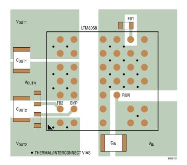
Figure 1. Layout Showing Suggested External Components, Planes and Thermal Vias
