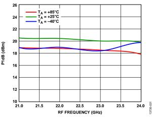
Figure 31. Output P1dB vs. RF Frequency at Various Temperatures, LO = 4 dBm
