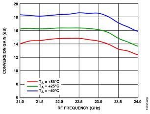
Figure 50. Conversion Gain vs. RF Frequency at Various Temperatures,  $LO = 4 \, dBm$
