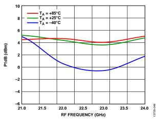
Figure 46. Input P1dB vs. RF Frequency at Various Temperatures, LO = 4 dBm
