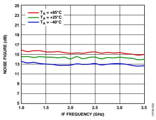
Figure 32. Noise Figure vs. IF Frequency at Various Temperatures, LO = 6 dBm, LO Frequency = 19 GHz
