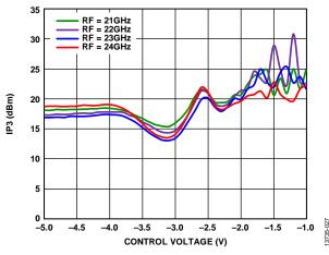
Figure 27. Input IP3 vs. Control Voltage at Various RF Frequencies,  $LO = 4 \ dBm$
