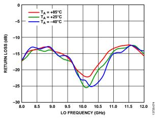
Figure 74. LO Return Loss vs. LO Frequency at Various Temperatures, LO = 4 dBm
