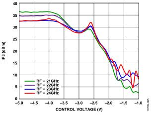
Figure 65. Output IP3 vs. Control Voltage at Various RF Frequencies, LO = 4 dBm
