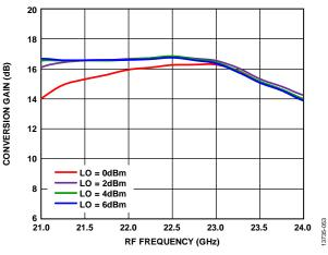
Figure 53. Conversion Gain vs. RF Frequency at Various LO Powers
