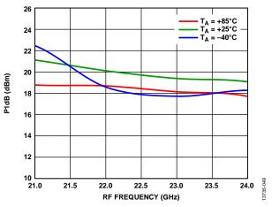
Figure 49. Output P1dB vs. RF Frequency at Various Temperatures,  $LO = 4 \ dBm$
