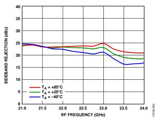
Figure 52. Sideband Rejection vs. RF Frequency at Various Temperatures, LO = 4 dBm
