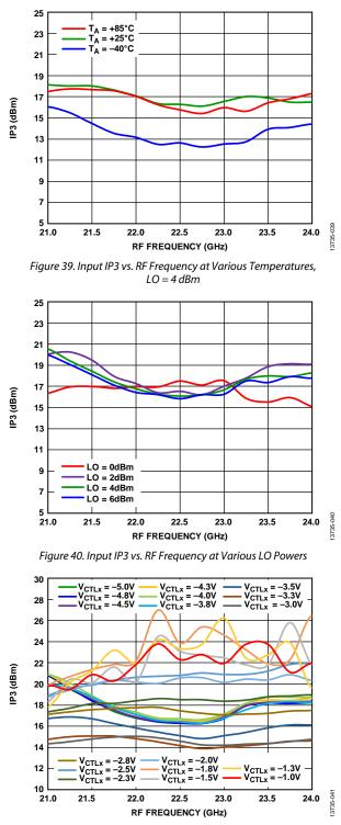
Figure 41. Input IP3 vs. RF Frequency at Various Control Voltages, LO = 4 dBm
