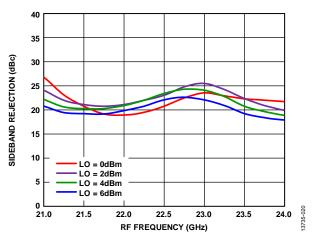
Figure 20. Sideband Rejection vs. RF Frequency at Various LO Powers
