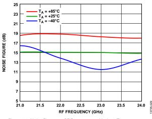
Figure 29. Noise Figure vs. RF Frequency at Various Temperatures, LO = 6 dBm
