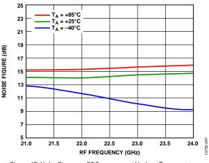
Figure 47. Noise Figure vs. RF Frequency at Various Temperatures, LO = 6 dBm
