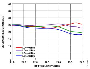
Figure 55. Sideband Rejection vs. RF Frequency at Various LO Powers
