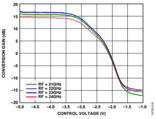
Figure 19. Conversion Gain vs. Control Voltage at Various RF Frequencies,  $LO = 4 \, dBm$
