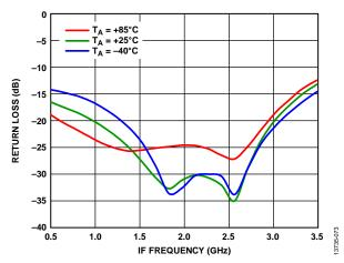
Figure 73. IF1 Return Loss vs. IF Frequency at Various Temperatures,  $LO = 4 \, dBm$  at LO Frequency = 20 GHz
