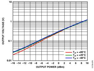
Figure 76. Detector Output Voltage ( $V_{REF} - V_{DET}$ ) vs. Output Power at Various Temperatures, LO = 17.5 GHz
