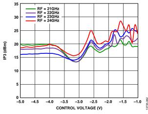
Figure 62. Input IP3 vs. Control Voltage at Various RF Frequencies,  $LO = 4 \ dBm$
