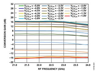
Figure 51. Conversion Gain vs. RF Frequency at Various Control Voltages,  $LO = 4 \ dBm$
