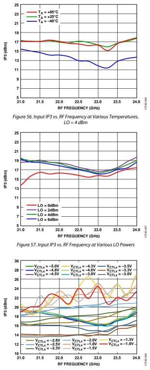
Figure 58. Input IP3 vs. RF Frequency at Various Control Voltages, LO = 4 dBm
