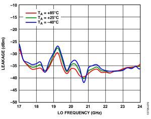
Figure 70. 2× LO Leakage at IF1 vs. LO Frequency at Various Temperatures,  $LO = 4 \, dBm$
