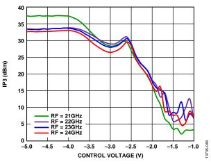
Figure 48. Output IP3 vs. Control Voltage at Various RF Frequencies, LO = 4 dBm
