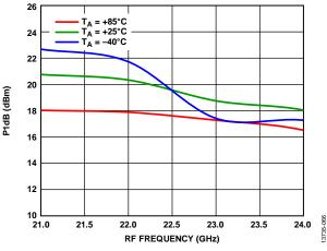
Figure 66. Output P1dB vs. RF Frequency at Various Temperatures, LO = 4 dBm
