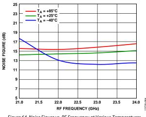
Figure 64. Noise Figure vs. RF Frequency at Various Temperatures,  $LO = 6 \ dBm$
