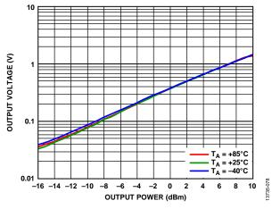
Figure 78. Detector Output Voltage ( $V_{REF} - V_{DET}$ ) vs. Output Power at Various Temperatures, LO = 20.5 GHz
