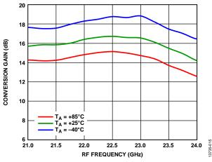
Figure 15. Conversion Gain vs. RF Frequency at Various Temperatures,  $LO = 4 \, dBm$
