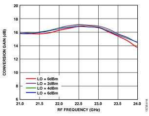
Figure 18. Conversion Gain vs. RF Frequency at Various LO Powers
