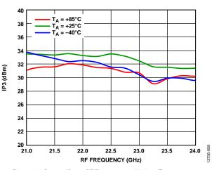
Figure 59. Output IP3 vs. RF Frequency at Various Temperatures, LO = 4 dBm
