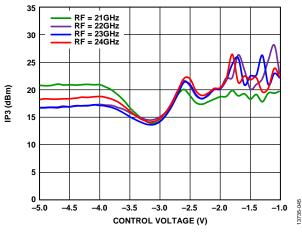
Figure 45. Input IP3 vs. Control Voltage at Various RF Frequencies,  $LO = 4 \ dBm$
