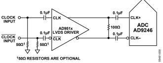
Figure 48. Differential LVDS Sample Clock
