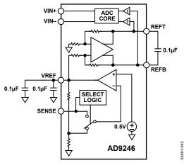
Figure 42. Internal Reference Configuration
