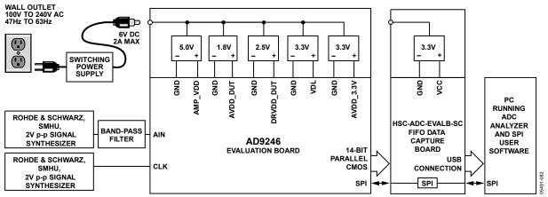
Figure 59. Evaluation Board Connection
