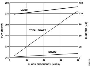
Figure 54. AD9246-80 Power and Current vs. Clock Frequency  $f_{IN} = 30$  MHz
