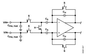
Figure 36. Switched Capacitor SHA Input
