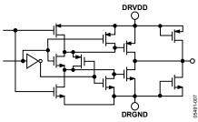
Figure 7. Equivalent Digital Output Circuit
