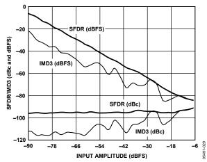
Figure 28. AD9246 Two-Tone SFDR/IMD vs. Input Amplitude (AIN) with  $F_{IN1} = 169.1$  MHz,  $F_{IN2} = 172.11$  MHz
