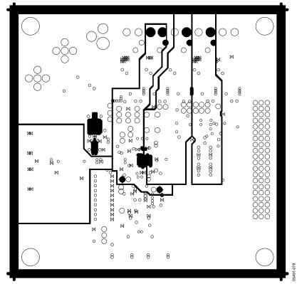
Figure 68. Evaluation Board Layout, Power Plane
