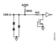
Figure 9. Equivalent CSB Input Circuit
