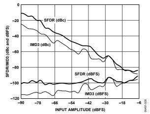
Figure 27. AD9246 Two-Tone SFDR/IMD vs. Input Amplitude (AIN) with  $F_{IN1} = 29.1 \text{ MHz}$ ,  $F_{IN2} = 32.1 \text{ MHz}$
