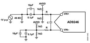
Figure 39. Single-Ended Input Configuration
