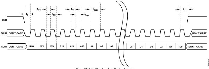
Figure 57. Serial Port Interface Timing Diagram
