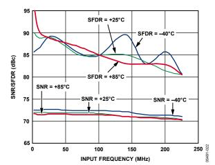
Figure 21. AD9246 Single-Tone SNR/SFDR vs. Input Frequency (f<sub>in</sub>) and Temperature with 2 V p-p Full Scale
