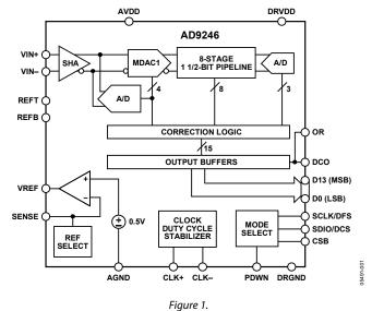
The digital output data is presented in offset binary, Gray code, or twos complement formats. A data output clock (DCO) is provided to ensure proper latch timing with receiving logic.
