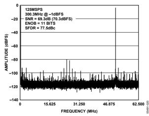
Figure 19. AD9246-125 Single-Tone FFT with  $f_{IN}$  = 300.3 MHz
