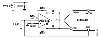
Figure 37. Differential Input Configuration Using the AD8138
