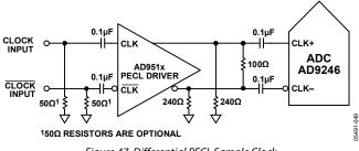
Figure 47. Differential PECL Sample Clock
