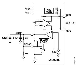
Figure 43. Programmable Reference Configuration
