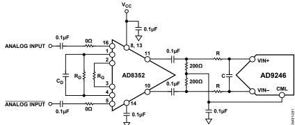
Figure 41. Differential Input Configuration Using the AD8352
