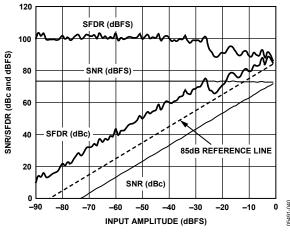
Figure 20. AD9246 Single-Tone SNR/SFDR vs. Input Amplitude (AIN) with  $f_{\rm IN}$  = 2.4 MHz
