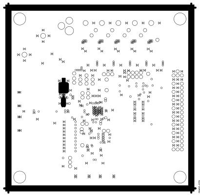
Figure 67. Evaluation Board Layout, Ground Plane
