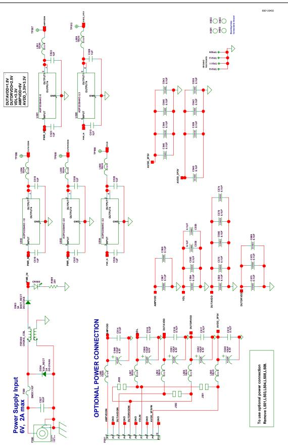
Figure 64. Evaluation Board Schematic, Power Supply Inputs
