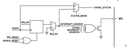
Figure 57. Simplified Schematic of IRQx Circuitry
