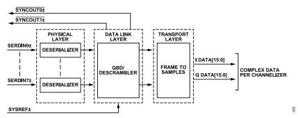
Figure 25. Functional Block Diagram of Serial Link Receiver
