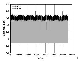
Figure 16. DNL, I<sub>OUTFS</sub> = 15.6 mA, 16-Bit Resolution
