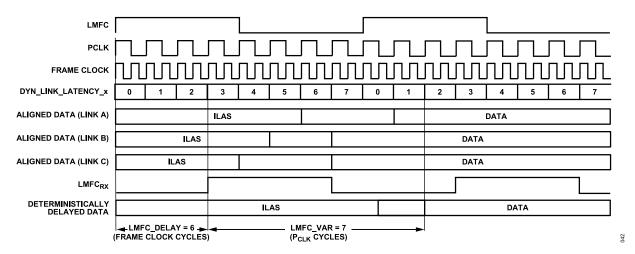
Figure 41. Multilink Synchronization Settings, Derived Method Example
