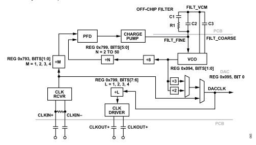
Figure 64. DAC PLL and Clock Path Block Diagram
