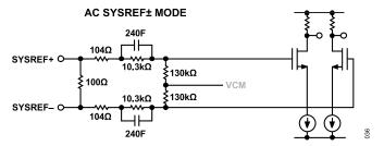
Figure 35. AC-Coupled SYSREF± Receiver Circuitry
