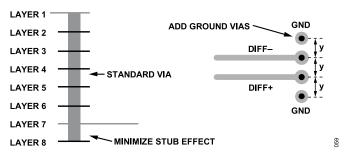
Figure 58. Minimizing Stub Effect and Adding Ground Vias for Differential Stripline Traces
