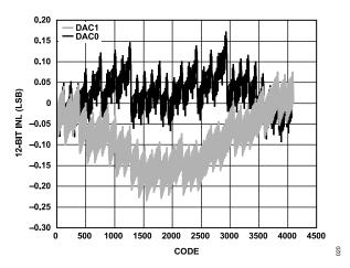
Figure 19. INL, I<sub>OUTFS</sub> = 20 mA, 12-Bit Resolution
