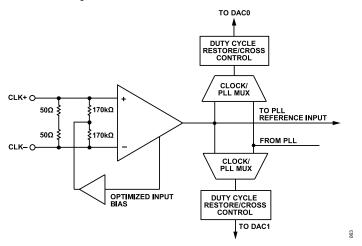
Figure 62. Clock Receiver Input Simplified Equivalent Circuit
