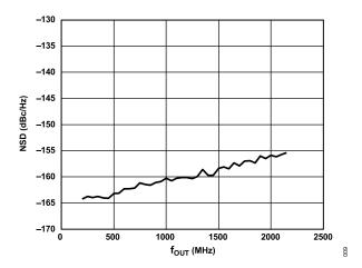
Figure 9. Single-Tone NSD Measured at 10% Offset from  $f_{\rm OUT}$  vs.  $f_{\rm OUT}$ ,  $f_{\rm DAC}$  = 5.89824 GHz, 16-Bit Resolution, Shuffle On
