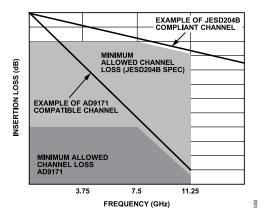
Figure 29. Insertion Loss Allowed
