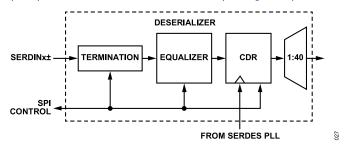
Figure 26. Deserializer Block Diagram
