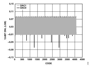
Figure 18. DNL, I<sub>OUTFS</sub> = 20 mA, 12-Bit Resolution
