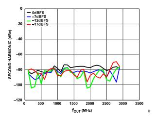
Figure 3. Second Harmonic (dBc) vs. f<sub>OUT</sub> over Digital Scale (Mode 0),6 GHz DAC Sample Rate, Channel Interpolation 2×, Main Interpolation 8×
