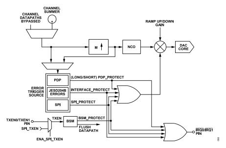
Figure 49. Block Diagram of Downstream Protection Triggers
