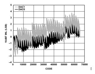
Figure 15. INL, I<sub>OUTFS</sub> = 20 mA, 16-Bit Resolution
