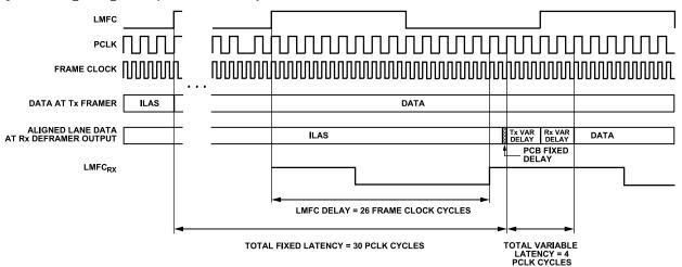
Figure 39. LMFC Delay Calculation Example
