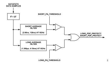
Figure 50. PDP Block Diagram
