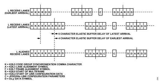
Figure 33. Lane Alignment During ILAS
