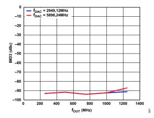
Figure 7. IMD3 vs. f<sub>OUT</sub> over f<sub>DAC</sub> (Mode 0), Channel Interpolation 2×, Main Interpolation 8×, 1 MHz Tone Spacing
