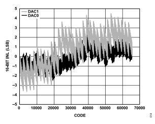
Figure 13. INL, I<sub>OUTFS</sub> = 26 mA, 16-Bit Resolution
