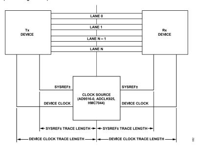
Figure 61. SYSREF± Signal and Device Clock Trace Length
