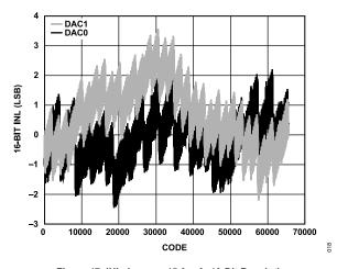
Figure 17. INL, I<sub>OUTFS</sub> = 15.6 mA, 16-Bit Resolution
