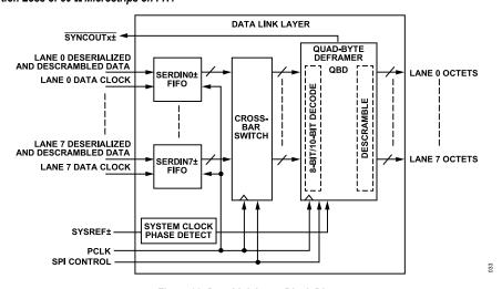
Figure 32. Data Link Layer Block Diagram
