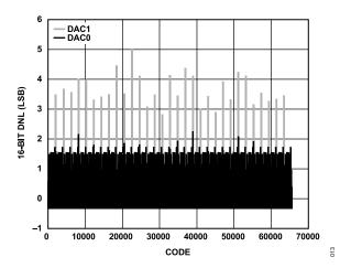
Figure 12. DNL, I<sub>OUTFS</sub> = 26 mA, 16-Bit Resolution
