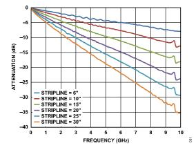
Figure 30. Insertion Loss of 50 Ω Striplines on FR4
