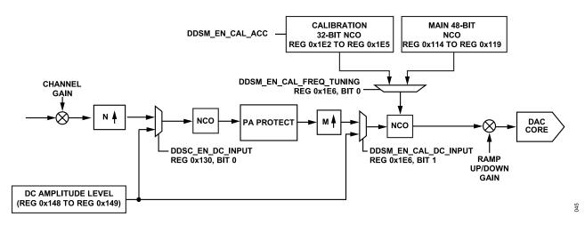
Figure 44. DC Amplitude Injection for NCO Only Mode Block Diagram
