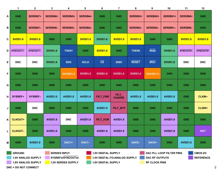
Figure 2. Pin Configuration
