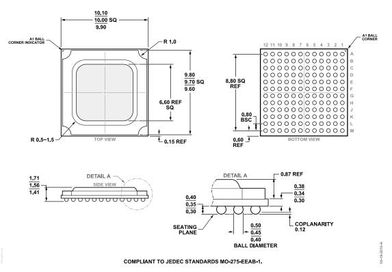
Figure 66. 144-Ball Ball Grid Array, Thermally Enhanced [BGA\_ED]
