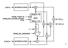
Figure 52. NCO Modulator Block Diagram
