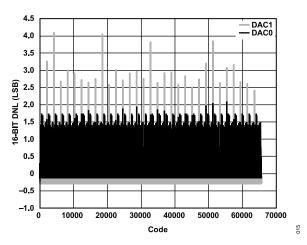
Figure 14. DNL, I<sub>OUTFS</sub> = 20 mA, 16-Bit Resolution
