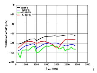
Figure 4. Third Harmonic (dBc) vs. f<sub>OUT</sub> over Digital Scale (Mode 0),6 GHz DAC Sample Rate, Channel Interpolation 2×, Main Interpolation 8×
