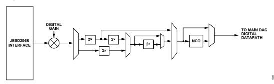
Figure 45. Block Diagram of the Channel Digital Datapath per the Main DAC Output
