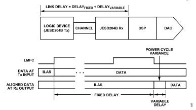
Figure 36. JESD204B Link Delay = Fixed Delay + Variable Delay
