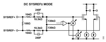
Figure 34. DC-Coupled SYSREF± Receiver Circuitry
