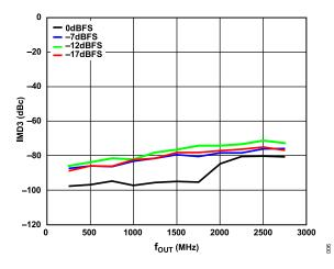
Figure 6. IMD3 vs. f<sub>OUT</sub> over Digital Scale (Mode 0) 6 GHz DAC Sample Rate, Channel Interpolation 2×, Main Interpolation 8×, 1 MHz Tone Spacing
