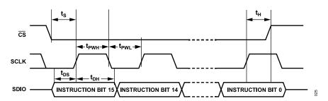
Figure 24. Timing Diagram for Serial Port Register Write
