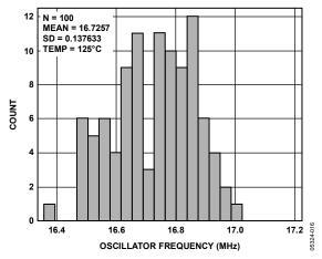
Figure 16. Frequency Distribution of Internal Oscillator at 125°C
