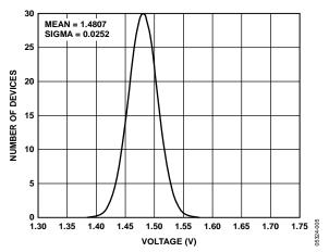
Figure 5. Range 1 DC Bias Distribution, VDD = 3.3 V
