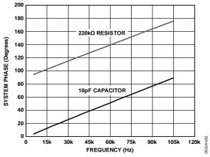
Figure 26. System Phase Response vs. Capacitive Phase
