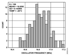
Figure 14. Frequency Distribution of Internal Oscillator at −40°C
