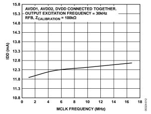
Figure 12. Typical Supply Current vs. MCLK Frequency
