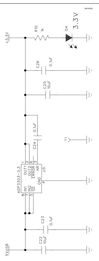
Figure 41. Linear Regulator on the EVAL-AD5933EB Evaluation Board
