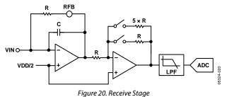
The digital data from the ADC is passed directly to the DSP core of the AD5933, which performs a DFT on the sampled data.
