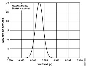
Figure 8. Range 3 Output Excitation Voltage Distribution, VDD = 3.3 V
