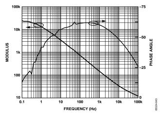
Figure 38. Bode Plot for Aluminum Corrosion Sensor
