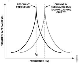
Figure 37. Detecting a Change in Resonant Frequency
