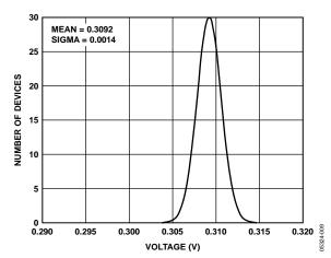
Figure 9. Range 3 DC Bias Distribution, VDD = 3.3 V
