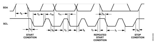
Figure 2. I<sup>2</sup>C Interface Timing Diagram
