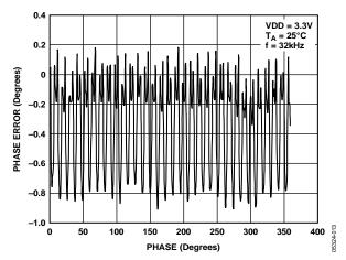
Figure 13. Typical Phase Error
