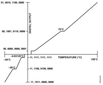
Figure 21. Temperature Sensor Transfer Function
