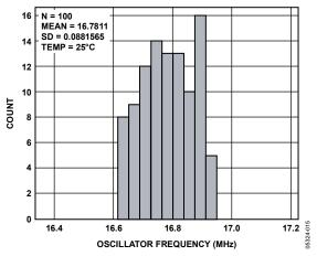
Figure 15. Frequency Distribution of Internal Oscillator at 25°C
