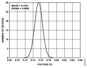
Figure 7. Range 2 DC Bias Distribution, VDD = 3.3 V
