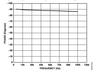
Figure 27. Phase Response of a Capacitor
