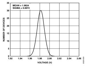
Figure 4. Range 1 Output Excitation Voltage Distribution, VDD = 3.3 V
