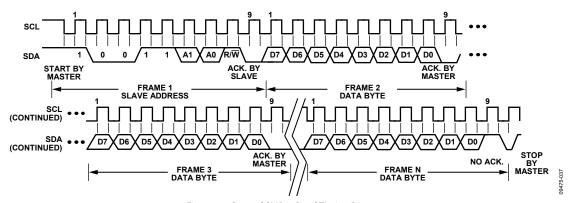
Figure 37. General SMBus Read Timing Diagram
