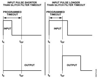
Figure 22. Input Glitch Filter Function
