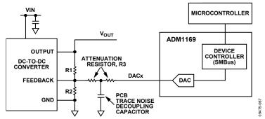
Figure 32. Open-Loop Margining System Using the ADM1169
