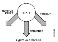
The ADM1169 offers up to 63 state definitions. The signals monitored to indicate the status of the input pins are the outputs of the SFDs.
