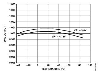
Figure 19. DAC Output vs. Temperature
