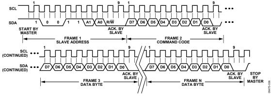
Figure 36. General SMBus Write Timing Diagram
