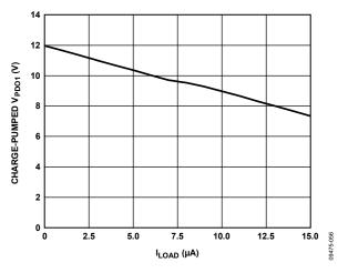
Figure 11. Charge-Pumped V<sub>PDO1</sub> (FET Drive Mode) vs. I<sub>LOAD</sub>
