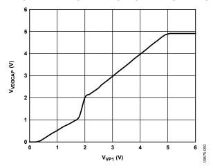
Figure 5. V<sub>VDDCAP</sub> vs. V<sub>VP1</sub>
