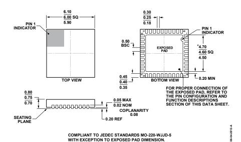
Figure 49. 40-Lead Lead Frame Chip Scale Package [LFCSP\_WQ] 6 mm × 6 mm Body, Very Thin Quad (CP-40-7) Dimensions shown in millimeters
