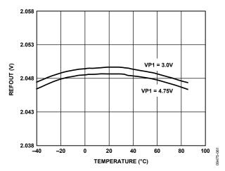
Figure 20. REFOUT vs. Temperature
