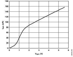
Figure 8. I<sub>VP1</sub> vs. V<sub>VP1</sub> (VP1 Not as Supply)
