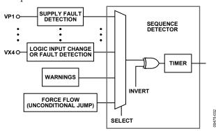
Figure 27. Sequence Detector Block Diagram
