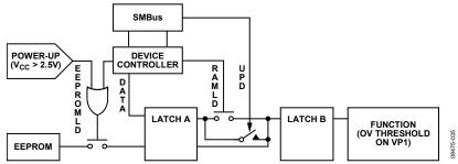
Figure 35. Configuration Update Flow Diagram
