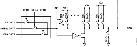
Figure 25. Programmable Driver Output
