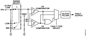
Figure 23. Supply Fault Detector Block
