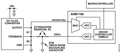
Figure 33. Closed-Loop Margining System Using the ADM1169
