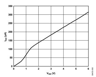
Figure 10. I<sub>VH</sub> vs. V<sub>VH</sub> (VH Not as Supply)
