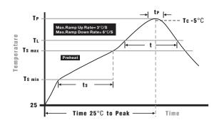
Wave Soldering:  $260^{\circ}\text{C}$ , 10 seconds max. Infrared Reflow: 260°C, 30 seconds max.
