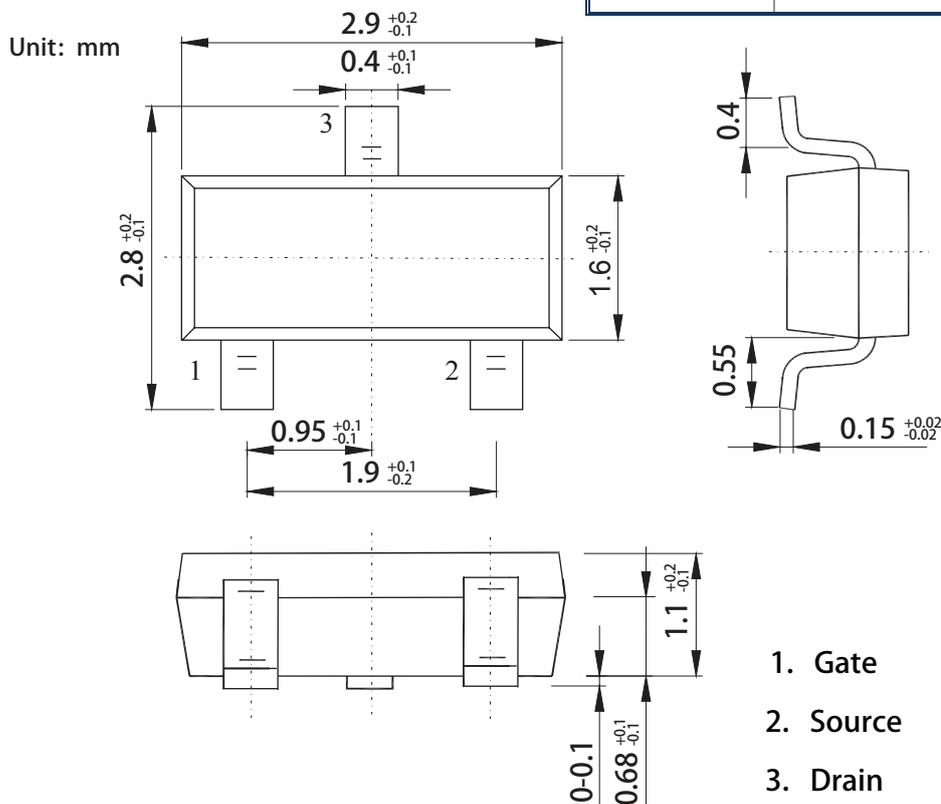
P-Channel Enhancement Mode Field Effect Transistor
