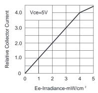
FIG.5 RELATIVE COLLECTOR CURRENT VS IRRADIANCE
