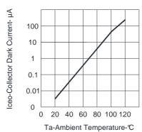
FIG.3 COLLECTOR DARK CURRENT VS AMBIENT TEMPERATURE
