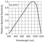
FIG.1 SPECTRAL SENSITIVITY
