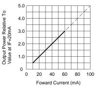
FIG.4 RELATIVE RADIANT INTENSITY VS. FORWARD CURRENT
