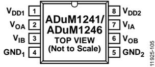
图7. ADuM1241/ADuM1246 8引脚SOIC (R-8)引脚配置
