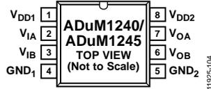
图5. ADuM1240/ADuM1245 8引脚SOIC (R-8)引脚配置
