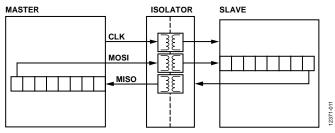
Figure 11. Standard SPI Configuration
