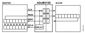
Figure 13. High Speed SPI Using Precision Clock Delay
