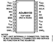
Figure 3. Pin Configuration
