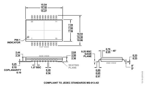
Figure 19. 20-Lead Standard Small Outline Package, with Increased Creepage [SOIC\_IC]
