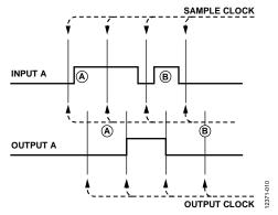
Figure 10. Low Speed Channel Timing
