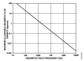
Figure 16. Maximum Allowable External Magnetic Flux Density
