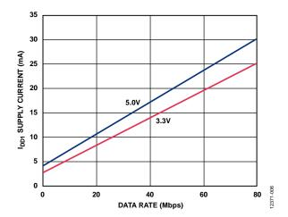
Figure 6. Typical  $I_{\text{DD1}}$  Supply Current vs. Data Rate for 5.0 V and 3.3 V Operation
