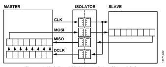
Figure 12. High Speed SPI Using Isolation Channel Delay
