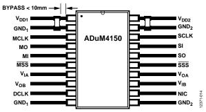
Figure 14. Recommended PCB Layout
