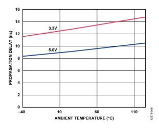
Figure 8. Typical Propagation Delay vs. Ambient Temperature for High Speed Channels Without Glitch Filter (See the High Speed Channels Section for Additional Information)
