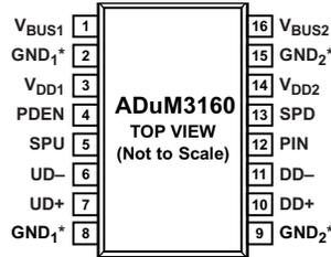
\*PIN 2 AND PIN 8 ARE INTERNALLY CONNECTED TO EACH OTHER, AND IT IS RECOMMENDED THAT BOTH PINS BE CONNECTED TO A COMMON GROUND.
