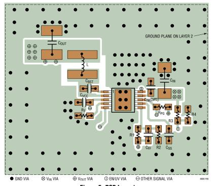
Figure 5. PCB Layout
