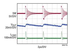
Figure 3. Burst Mode Operation
