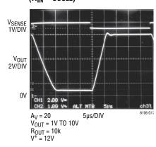
Step Response 0mV to 500mV ( $R_{IN} = 500\Omega$ )
