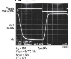
Step Response 10mV to 100mV  $(R_{IN} = 100\Omega)$
