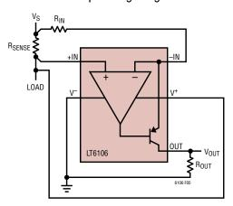
Figure 5. LT6106 Supply Current Monitored with the Load
