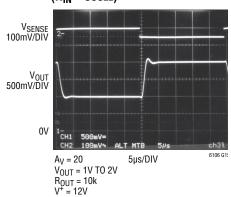
Step Response 0mV to 50mV ( $R_{IN} = 500\Omega$ )
