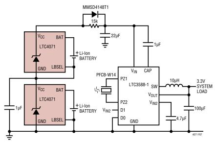
Figure 7. Piezoelectric Energy Harvester with Battery Backup
