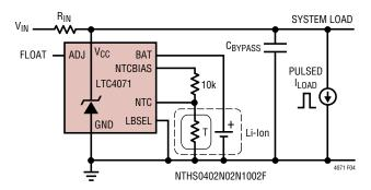
Figure 4. Adding a Decoupling Capacitor for Large Load Transients
