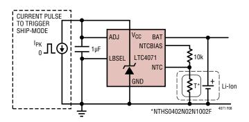
Figure 8. LTC4071 Ship-Mode Application for Extended Shelf Life
