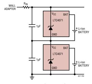
Figure 3. 2-Cell Battery Charger
