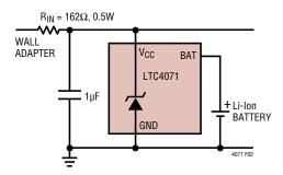
Figure 2. Single-Cell Battery Charger
