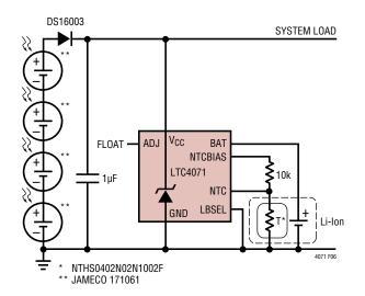
Figure 6. Simple Photovoltaic Charger
