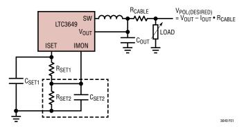
Figure 1. Cable Drop Compensation Application
