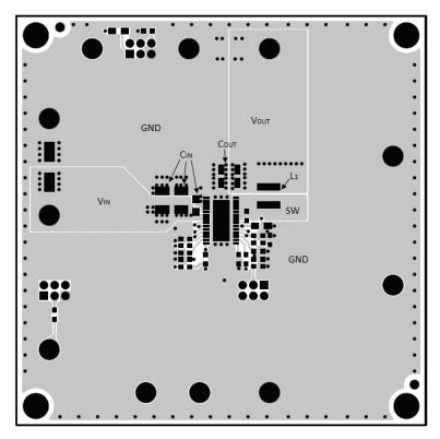
Figure 5. Sample PCB Layout
