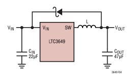
Figure 4. Schottky Diode from V<sub>OUT</sub> to V<sub>IN</sub>
