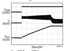
$\begin{array}{l} V_{IN} = 24V, \, R_{ISET} = 100k\Omega \\ R_{LOAD} = 10\Omega, \, L = 2.2\mu H \, R_{ITH} = 4k\Omega, \\ C_{ITH} = 2.2nF, \, C_{ITHP} = 47pF, \, R_{IMON} = 40k\Omega, \\ C_{IMON} = 0.47nF, \, C_{OUT} = 2\times 47\mu F + 36mF \end{array}$
