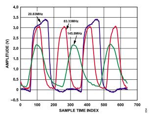
Figure 22. SYNC\_CLK Amplitude at Various Frequencies (f<sub>SYSCLK</sub>/24), Measured at the SYNC\_CLK Pin Using an Active Probe (1 GHz Bandwidth, 1 MΩ, 1 pF) with the SYNC\_CLK Pin Loaded by a 1-inch PCB Trace Connected to an Open SMA Connector
