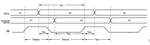
Figure 48. Parallel Port Write Timing Diagram
