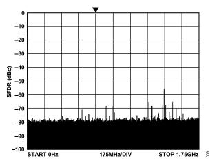
Figure 6. Wideband SFDR at 696.5 MHz, SYSCLK = 3.5 GHz (SYSCLK PLL Bypassed)
