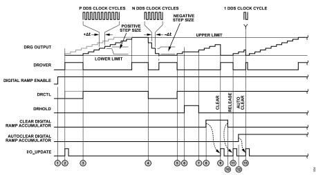
Figure 39. Normal Ramp Generation
