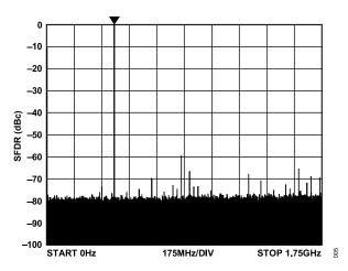
Figure 5. Wideband SFDR at 427.5 MHz, SYSCLK = 3.5 GHz (SYSCLK PLL Bypassed)
