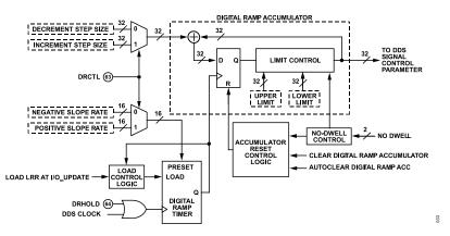
Figure 38. Digital Ramp Generator Detail
