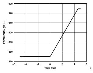
Figure 25. Measured Rising Linear Frequency Sweep
