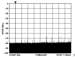
Figure 4. Wideband SFDR at 171.5 MHz, SYSCLK = 3.5 GHz (SYSCLK PLL Bypassed)
