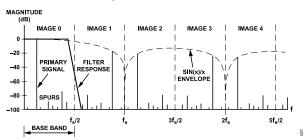
Figure 32. DAC Spectrum vs. Reconstruction Filter Response
