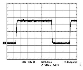
Figure 23. SYNC\_OUT (f<sub>SYSCLK</sub>/384)
