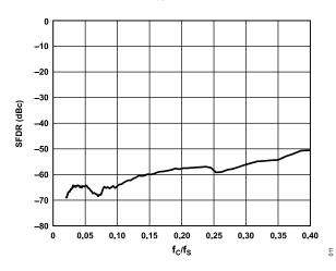
Figure 11. Wideband SFDR vs. Normalized f<sub>OUT</sub>, SYSCLK = 3.5 GHz
