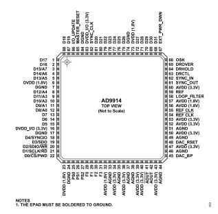
Figure 3. Pin Configuration
