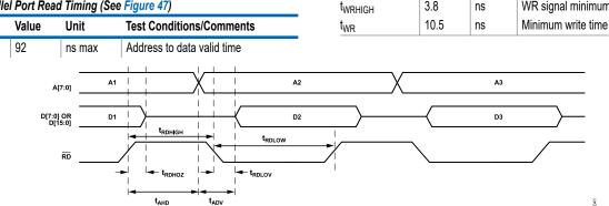
Figure 47. Parallel Port Read Timing Diagram
