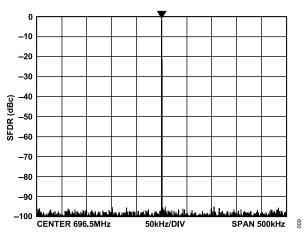
Figure 9. Narrow-Band SFDR at 696.5 MHz, SYSCLK = 3.5 GHz (SYSCLK PLL Bypassed)
