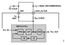
Figure 35. REF CLK PLL External Loop Filter
