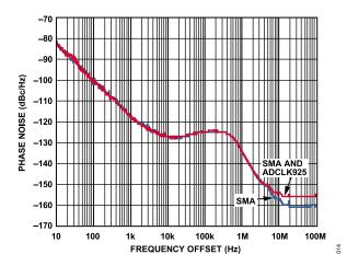
Figure 14. Absolute Phase Noise of REF CLK Source (Rohde & Schwarz SMA100 Signal Generator at 3.5 GHz Buffered by Series ADCLK925) Driving AD9914
