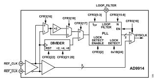
Figure 33. REF\_CLK Block Diagram
