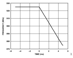
Figure 26. Measured Falling Linear Frequency Sweep
