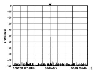
Figure 8. Narrow-Band SFDR at 427.5 MHz, SYSCLK = 3.5 GHz (SYSCLK PLL Bypassed)
