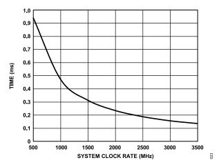
Figure 24. DAC Calibration Time vs. SYSCLK Rate. See the DAC Calibration Output Section for Formula.
