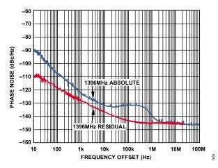
Figure 20. Residual PN vs. Absolute PN Measurement Curves at 1396 MHz
