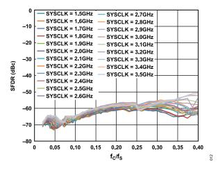
Figure 12. Wideband SFDR vs. Normalized f<sub>OUT</sub>, SYSCLK = 1.5 GHz to 3.5 GHz
