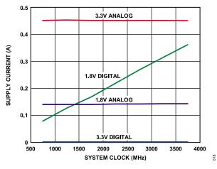
Figure 18. Power Supply Current vs. SYSCLK
