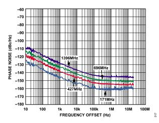
Figure 17. Residual Phase Noise Curves
