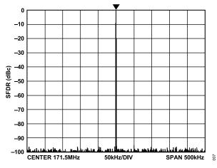
Figure 7. Narrow-Band SFDR at 171.5 MHz, SYSCLK = 3.5 GHz (SYSCLK PLL Bypassed)
